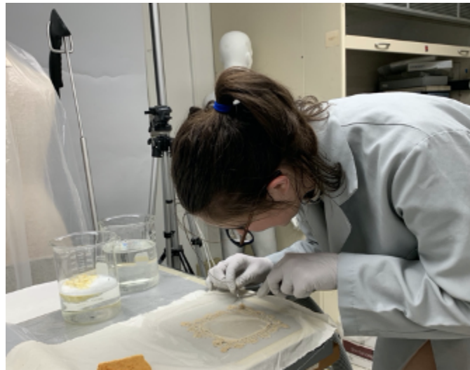
Diane Walker positioning a textile with a tatting border on a suction table for cleaning in the FIT wet lab.
