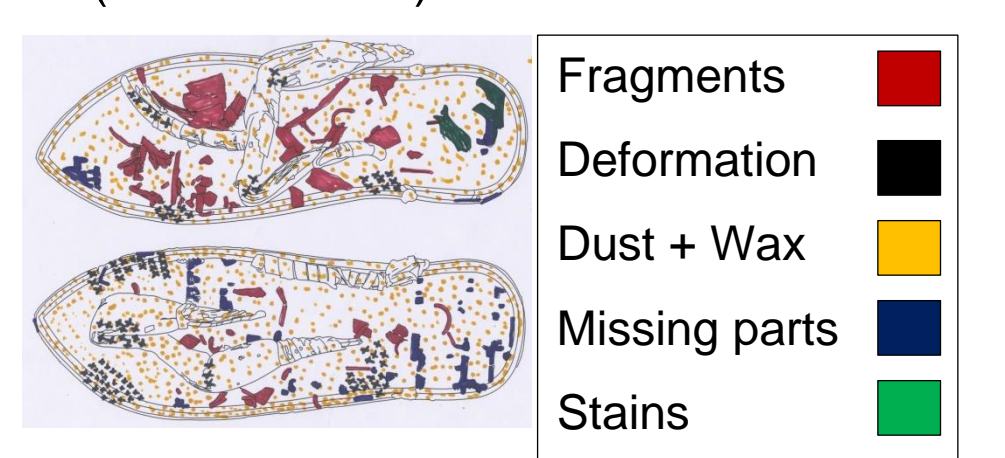
Deterioration map with AutoCAD 2D.
